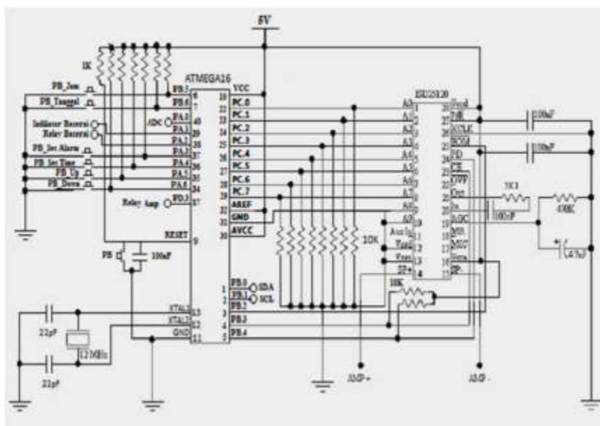
Gambar 4 Rangkaian Dot Matrix LED
